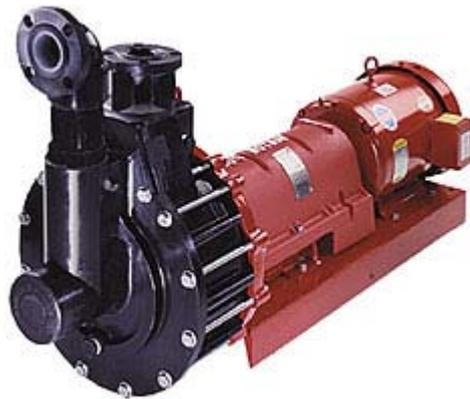
As with all Vanton thermoplastic pumps, no metal components are in contact with the fluid being handled. Even the large diameter steel shaft is isolated from the fluid by a thick sectioned thermoplastic sleeve. No metallic contamination is possible.
